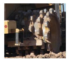
**Cleaner Bars.** Help keep the drums free of carry-over dirt regardless of rolling direction. A pass-through bolt design allows for easier serviceability.
