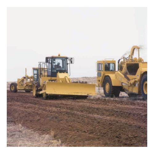
**Blade Package.** Consists of the blade, push-arms, trunnion mounting, dozerlength skid plate with replaceable wear plates, reversible cutting edges, selfsharpening end bits, hydraulic lines guard and hydraulic lift cylinders. **Operator Controls.** The tilt cylinder is an option that gives the 815F Series 2 more versatility when dozing. The controls are seat-mounted and located in a convenient location to the right of the operator.
