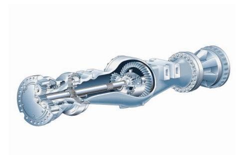
**Front Axle.** Is rigidly mounted to the frame to support the weight of the compactor, internal torque loads and external loads applied during compacting and dozing operations.
