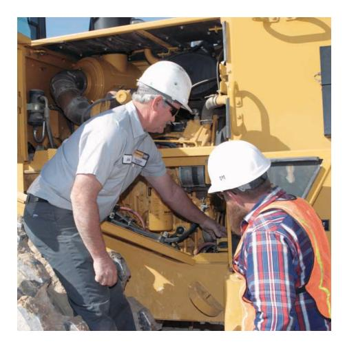
**Engine Access.** All metal engine enclosure and hinged access doors allow for easy daily maintenance and inspection.
